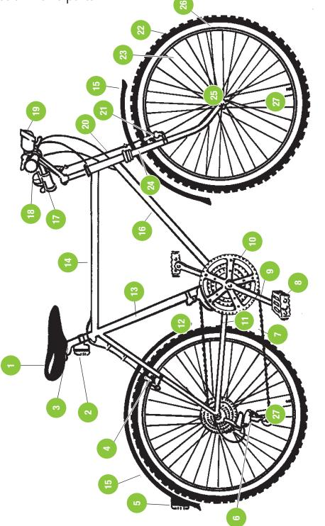
1 Seat 2 Rear light 3 Seat stay 4 Rear calliper brake 5 Red rear reflector 6 Rear derailleur 7 Chain 8 Pedal 9 Crank arm 10 Chain ring 11 Chain stay 12 Front derailleur 13 Seat tube 14 Top tube 15 Fenders 16 Down tube 17 Handlebar grip 18 Bell 19 Front light 20 Brake cable 21 Front calliper brake 22 Tire 23 Spokes 24 Fork 25 Hub 26 Rim 27 Tire valves
